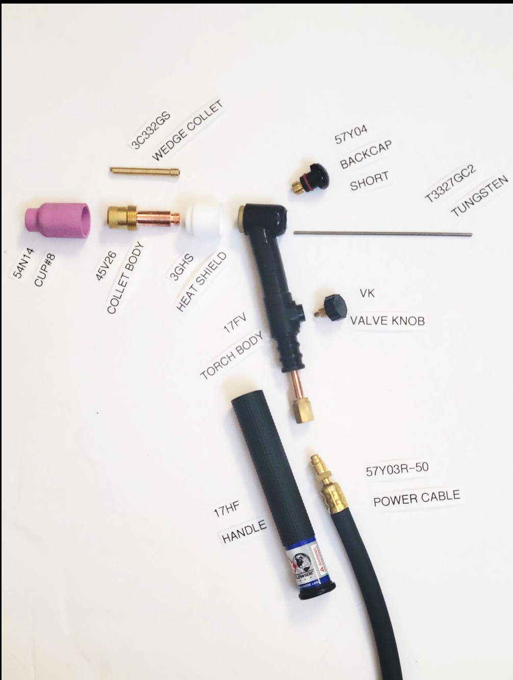
TIG Torch Gas/Power Assembly Part Diagram
